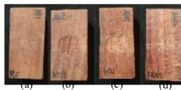
FIGURE 5. Deterioration pattern of acacia wood in green MC (a), 40-45% MC (b), Air-Dry MC (c), and Kiln-Dry MC (d).
